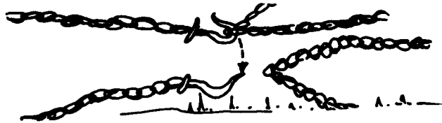
Figure L-14. USE OF HOOKS.
