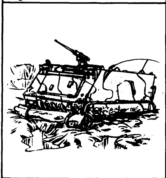
Figure L-8. MIRED APC RECOVERY.
